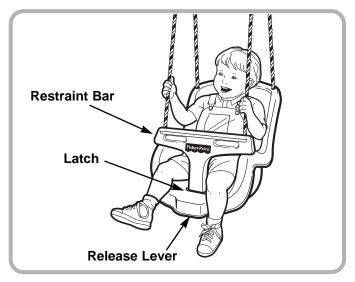
Insert the restraint bar down into the latch until it snaps into place. Pull up on the restraint bar to be sure it is securely latched.
